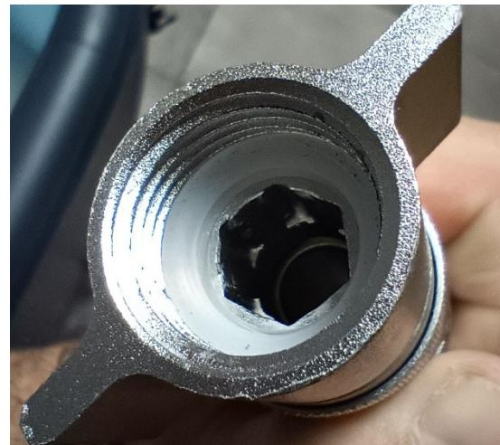
**Connect Hoses:** Hand Tight is acceptable, do not overtighten connections as this may strip the threads.
