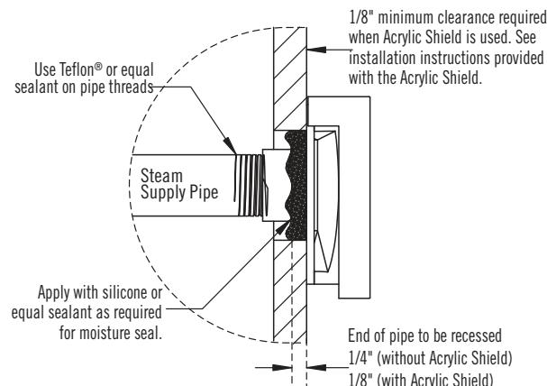
**CAUTION** Consult with supplier of acrylic, fiberglass and other non-heat resistant enclosures for recommended steamhead location. Use Acrylic Shield PN 103938/103938SQ. See instructions provided with steam shield. (An acrylic shield is not available for the iSteam steamhead.)
