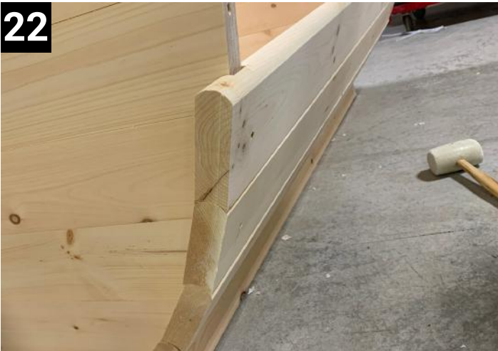
Put a total of 4 staves on each side now and fasten into wall
