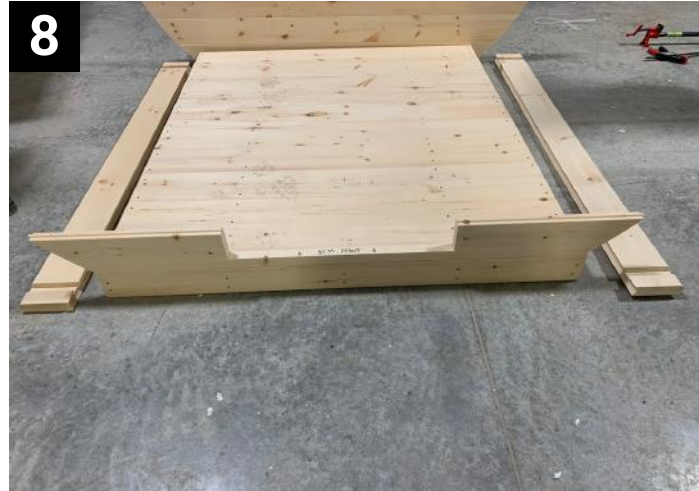
8 Lay front wall door pc on floor
